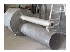
Midwest Tank Co. built this tank for the United Children's Hospital for chemical run-off. It is designed to be water tight and does not contain pressure. This is a buried tank with an 8 inch stainless steel pipe that runs parallel th the 24" dia access way. This picture shows a tank with a commercial blast on the exterior and a near white blast interior. The interior was lined with a Plasite 3066 and baked to the proper temp and time. The exterior was coated with coal tar epoxy.
