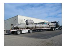
This is a Transporter tank we built in the hydro test stage. The tank is designed for transporting dry goods from one place to another. Midwest tank can build sizes from 24" to 96" diameter.
