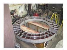
This is a Vibration Damper in the process of being built for a coal plant smoke stack.
