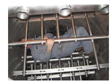
Midwest Tank Co. does not design systems. We build tanks to meet the customers design criteria for the vessel. This tank is an example of a complicated internal process that was manufactured to meet our customers | needs. As you can see, the entire tank was made of stainless as well as the internal piping system.
