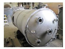
This cooling water tank is made of 316L and is designed for atmospheric pressure. The top and bottom rings are to hold insulation to be installed in the field. This is a vertical tank with 304L stainless steel legs.
