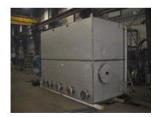
Midwest Tank Co. is not limited to building round tanks. The rectangular tank you see in this picture is undergoing a hydro-test. We test every tank prior to shipping to guarantee a quality tank. This tank was design with internal structures to keep the wall of the vessel from excessive deflection. The inside of this vessel has an internal screen to keep debris from entering the pumps and causing a shutdown of the system. The tank is made of 304L stainless. The exterior has a mill finish.
