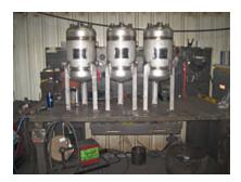
Small ASME Code pressure vessels made of 304L stainless steel with 3 angle legs for vertical mounting. These small stainless tanks were used as process tanks. The exterior of the tanks were finished with a white epoxy coating.
