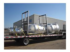
This photo has 3 stainless steel ASME pressure vessels that are used as flash tanks and process tanks for the ethanol industry. The tanks provide a longer life span than a carbon steel tank that may have been used in a similar situation. The exterior of these tanks are glass bead blasted.
