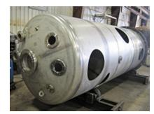
This vertical flash tank is made with 304L stainless and designed as an ASME pressure tank rated for 30 PSI and full vacuum. It has an internal baffle and contains (2)  $24^{\circ}$  dia. manholes for access. On the top of the tank are (2)  $6^{\circ}$  view ports installed for inspecting the inside of the tank while the tank is operating. The ring base is made of carbon steel and will be prime painted inside and out prior to shipping.
